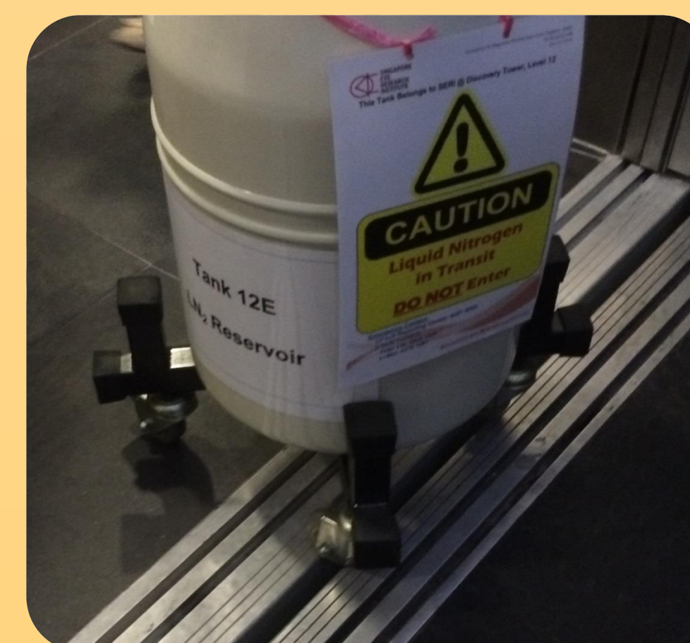
Lift gaps were measured to be 3cm. When tested, wheels size of less than 7cm were prone to getting trapped and had to be lifted to bypass the gap.
