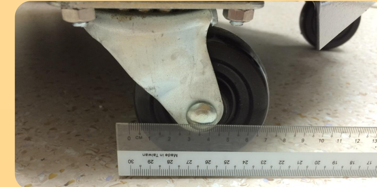
Of the 41 wheel size measured, 88% of the wheels were \leq 7 cm
