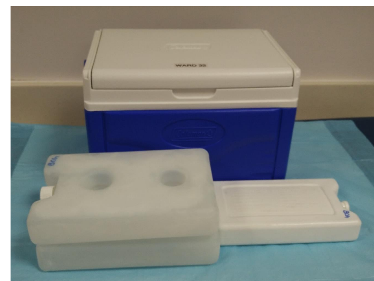
Two fully frozen ice packs (19 x 10.5 x 3cm) and one (18.5 x 9.5 x 2.5cm) are used to maintain cold chain
