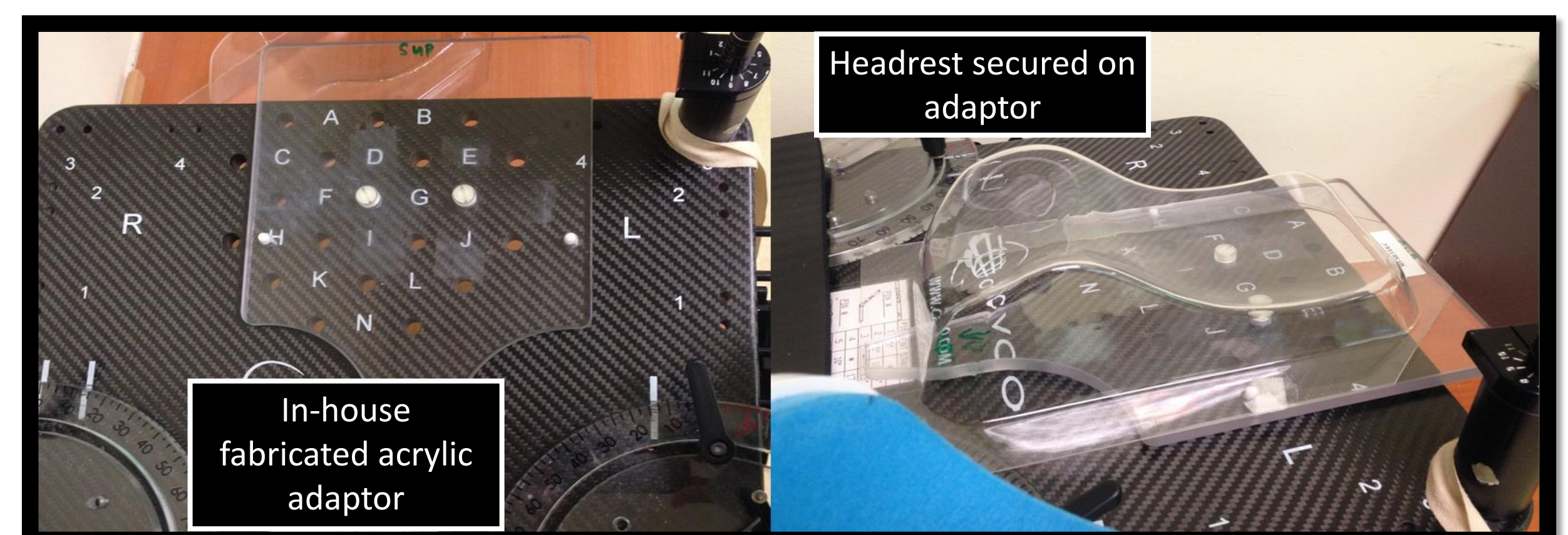
Intervention 3: Acrylic adaptor to secure headrest
