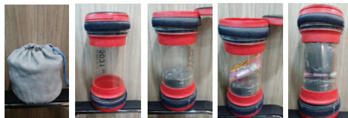
Fig. 4 A summary of how the blood tubes are being transported in the pneumatic tube "sandwiched" in between the specially designed sponge.
