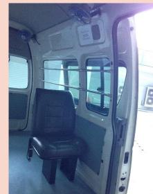
A grab bar was installed near the passenger's door for patients to hold on to and maintain their balance while boarding or alighting the ambulance.
