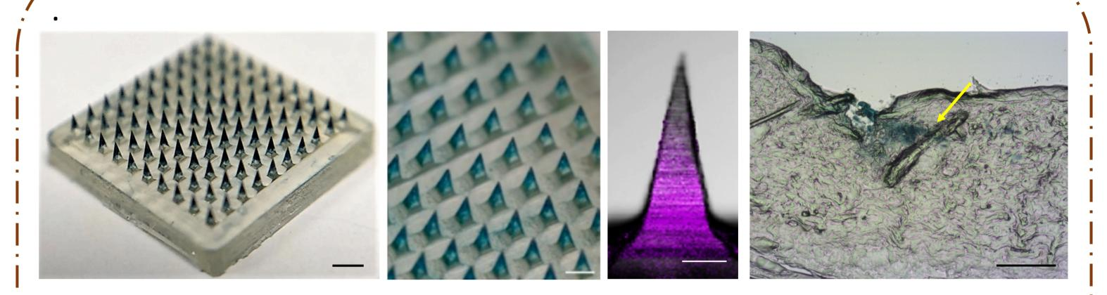
Microneedles are fabricated to 150-200µm using biocompatible and biodegradable polymers to ensure painless penetration of the oral epithelium without contacting nerve endings in the lamina propria.
