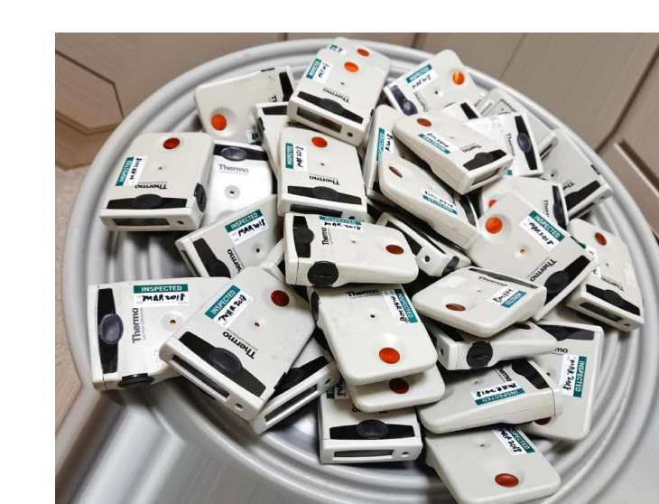
Figure 4: Radiation levels at 1m and 1.5m were measured using Thermo Mk2 electronic personal dose meters. These meters were calibrated to measure body dose in units of Sieverts. 5 dose meters were used for each distance and material.
