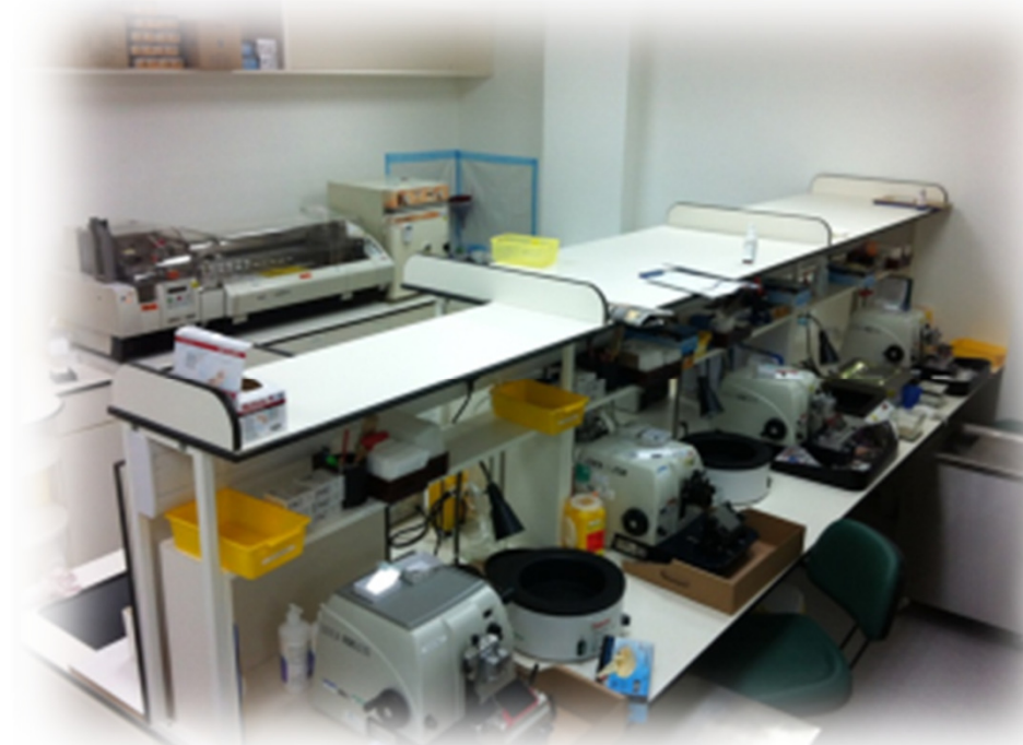
6 microtomes are now able to fit on the bench with orientation that eases the workflow
