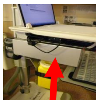
(1) Drawer was designed and fabricated between keyboard and the COW table top.
