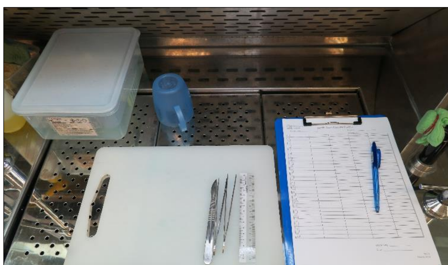
Organization of the work area to avoid clutter, minimize risk of mistakes.
