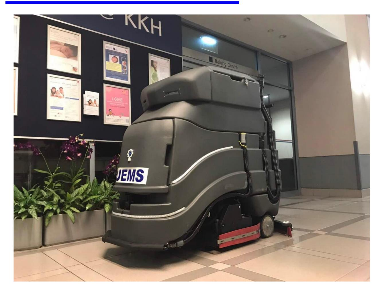
The autonomous Scrubber/Dryer is programmed to act on its own, independent of any controller. Its Technology is adopted from the robotics industry to enhance productivity for the cleaning industry.
