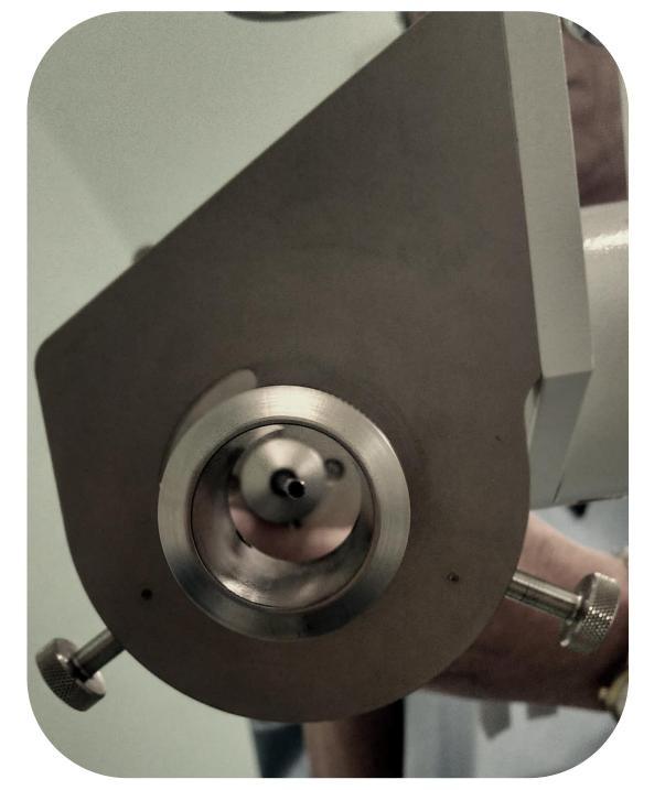
The current mounting process is done freehand by a handler. To maintain the mechanical straightness of the probe and prevent it from coming into contact with the suspension system, the handler needs to have stable hands, experience in handling the weight and a good estimate of the angle for entry. These factors vary with each individual handling the XRS.
