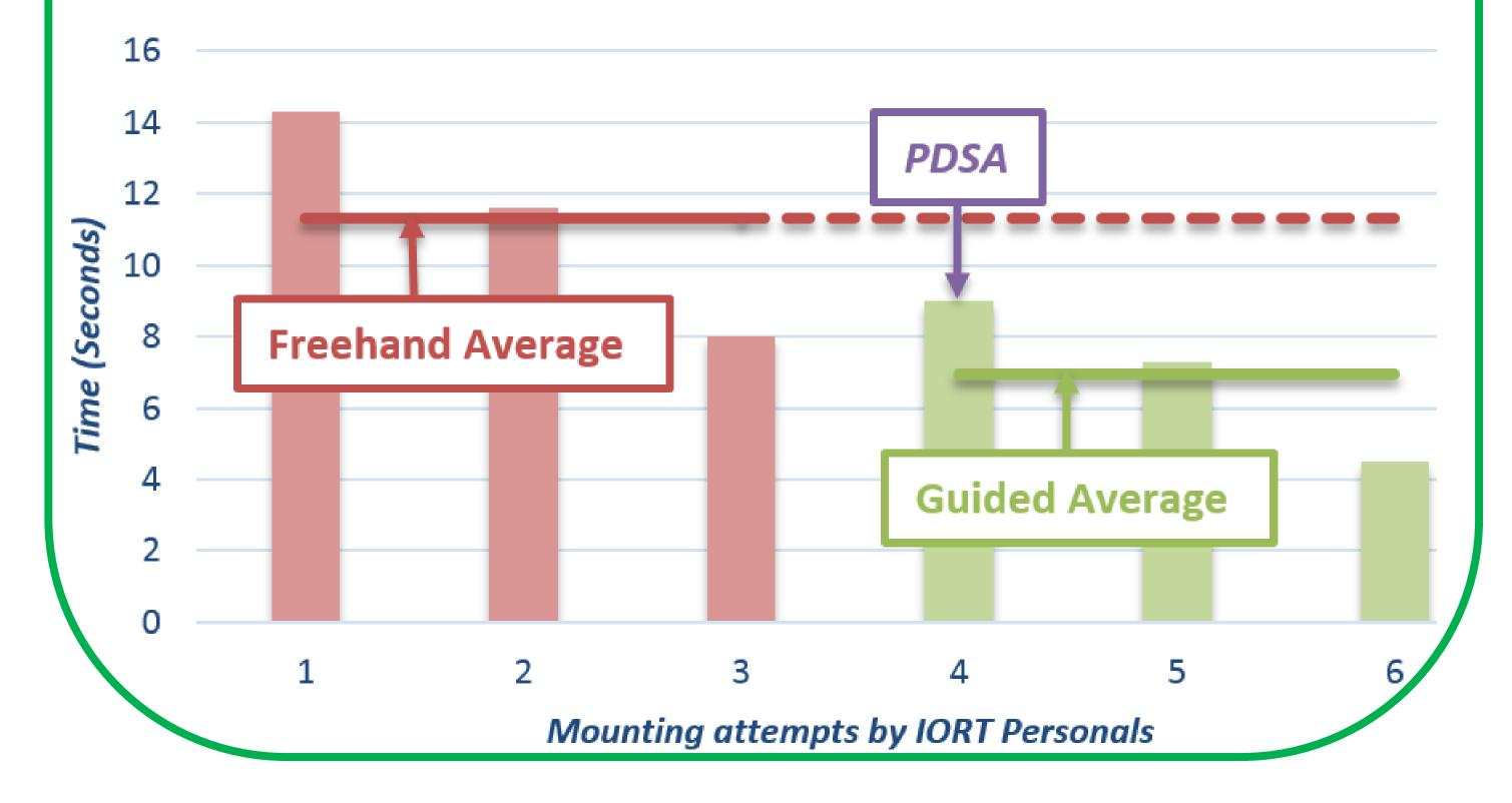
Radiation Therapist, Radiation Physicist, and Technician is formed to take on this challenge to reduce the variables caused by different handlers. A transparent Acrylic Guide for the XRS is designed and manufactured by the Technician. The time taken by 3 different handlers is recorded before and after using the Acrylic Guide to measure their mounting speed for comparisons.
