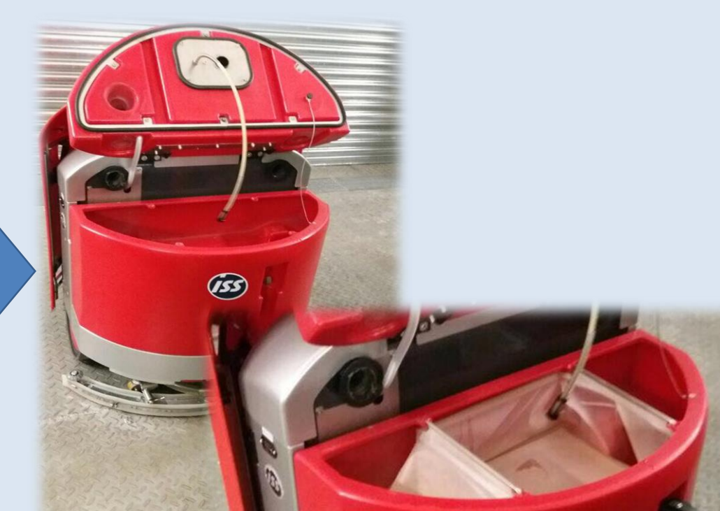
Water tank are emptied after cleaning complete.
