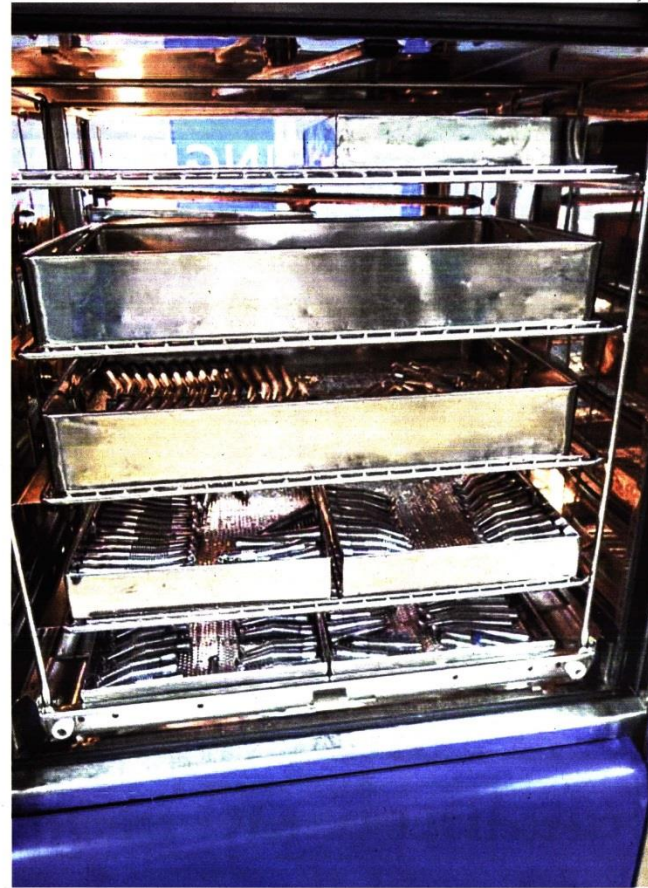
The first two steps of the sterilisation process take place in a thermal disinfectant, where dental instruments are washed and then thermally disinfected through a process that removes close to 100 per cent of organisms. Thermal disinfection takes place at 90 deg C for five minutes. PHOTO: NATIONAL DENTAL CENTRE SINGAPORE
