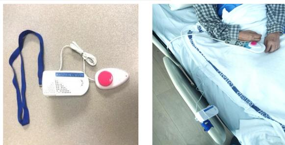
PDSA 1 started off with having a small foam added above the door bell to create a protruding surface that indirectly sounds off the alarm when triggered.
