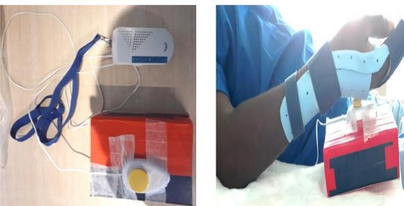
PDSA 2 added a securing function using clean recycled boxes to keep the modified call bell within reach. Nurses were briefed on how to adjust volume of modified call bell accordingly.
