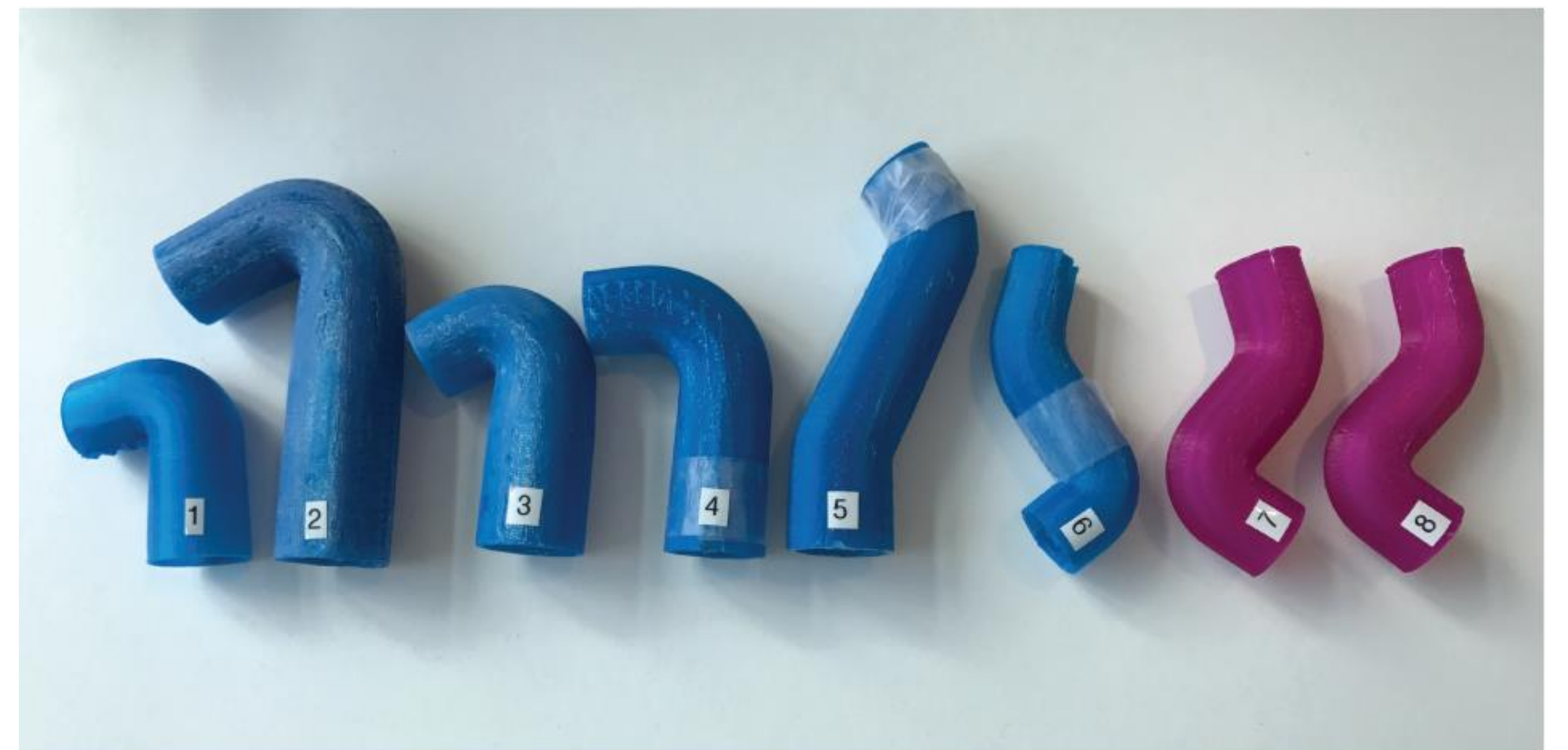
3D Printed Prototypes For The Study Of Optimum Angle.
